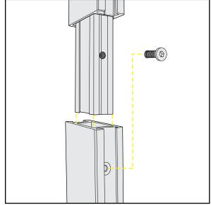
Inline Connection between Extrusions
