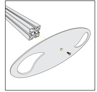
Baseplate Connection for Vertical Extrusions
