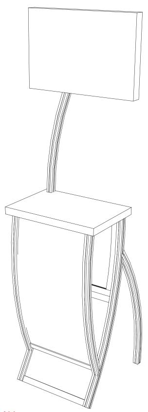
WHEN DISASSEMBLING ALUMINUM EXTRUSION, TIGHTEN ALL SETSCREWS AND LOCKS TO PREVENT LOSS DURING SHIPPING
