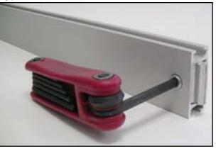
Detail A: Most horizontal extrusion connections have a patented expandable lock. This lock inserts into the groove of an opposing extrusion. Tightening the lock with the Hex Key Tool expands the lock and creates a strong positive connection.
