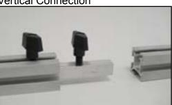
Detail E: A square connection bar with plastic T Knobs is inserted between two vertical extrusions joined end-to-end. Turn the knobs clockwise to tighten.
