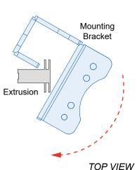
Slide bracket forward, then down onto V4 connector.
