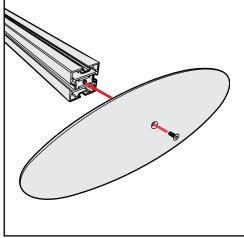
**Base Plate & Extrusion Connection**
