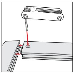
**Extrusion & Lock Connection**
