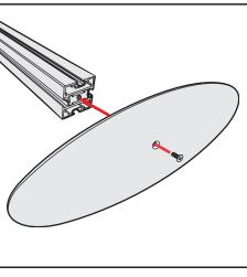
Base Plate & Extrusion Connection
