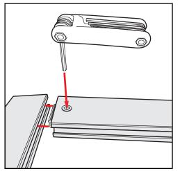
Extrusion & Lock Connection
