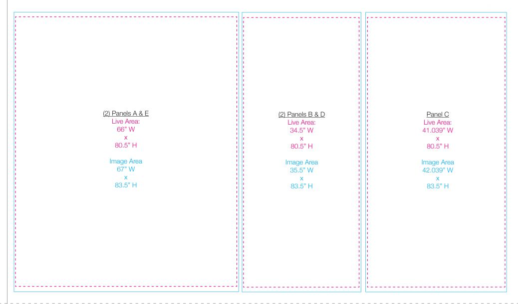
**NOTE:** Dimensions above are for full height panels with Velcro sewn to FRONT perimeter. Horizontal extrusion will be exposed. If it is preferred to hide horizontals, panel heights should be increased to 86.5" to account for 1.25" of live area on top and bottom that will wrap around the extrusion.
